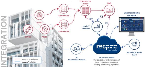
respira® is able to integrate in different ways depending on the existing BMS and the established requirements. It can be deployed as a system in the cloud or via Edge Computing and integrated through API or web server, database servers or directly into the communication protocol layer (OPC, Modbus, Bacnet, ...)
